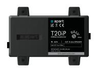
The T20IP is a small built-in 100 volt line transformer, designed to make it possible to convert a standard 8 ohms loudspeaker into a 100 volt line speaker with selectable power taps (2.5-5-10 and 20 watts in 100 volt).
