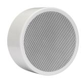
The Apart EN-SM6T10-W is a surface mounted speaker made of powder coated steel (RAL 9010 equivalent), equipped with a high efficiency full range speaker and a multi tap 100 volt transformer, all certified according EN 54-24. The unit is equipped with a ceramic speaker line connector block and thermal fuse.
